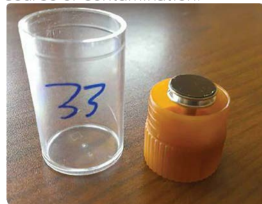
Example of a stub used for collection
