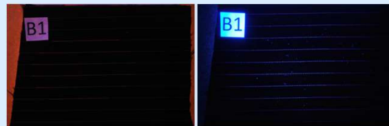
Figure 2. Sample B1 viewed with a Nova light (455nm) with an orange filter (left) and a UV LED light (right)
