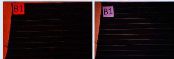
Figure 3. Sample B1 viewed with a laser light (532nm) with an orange filter (left) and an Astra light (455nm) with an orange filter (right)
