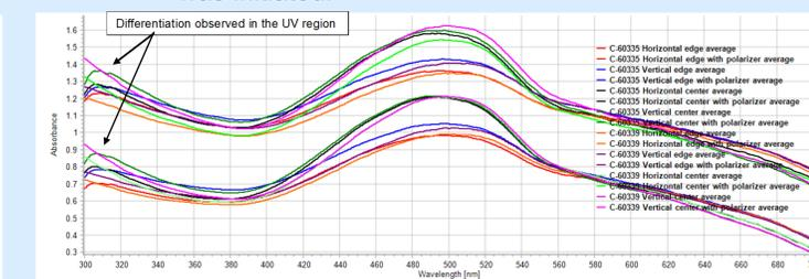
Figure 4: UV-Vis spectra showing differentiation of Samples C-60335 v. C-60339 with polarizer
