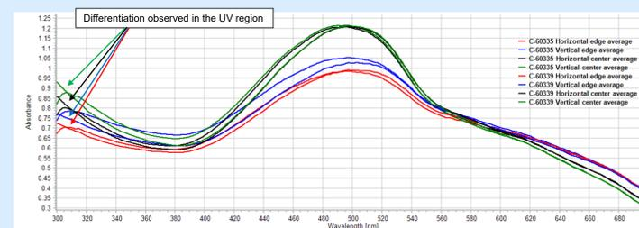
Figure 3: UV-Vis Spectra showing differentiation of Samples C-60335 v. C-60339
