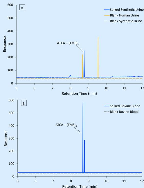
Figure 2: Overlaid extracted ion chromatograms (EIC) of ATCA - (TMS)<sub>3</sub> at 245, 347, and 362 m/z in (A) a blank synthetic urine, synthetic urine spiked with 1000 ng/mL ATCA only, and a human urine sample, and (B) a blank bovine blood and bovine blood sample spiked with 1000 ng/mL ATCA only.
