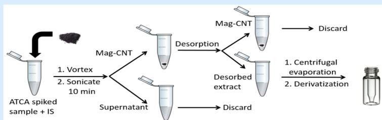
Figure 1: Simplified optimized Mag-CNT/d- $\mu$ SPE-GC/MS procedures.
