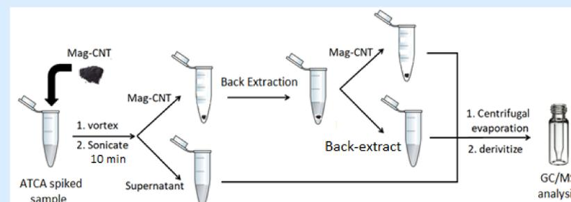
Figure 1: Simplified Mag-CNT/d-SPE-GC/MS procedures.
