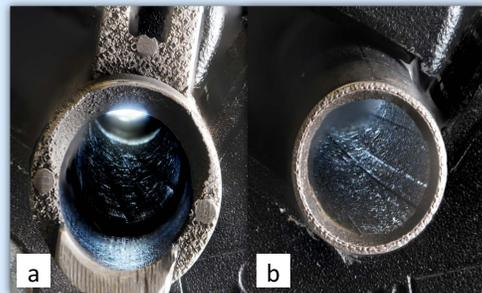
Figure 3: The close-up image of barrel A at the (a) chamber end and (b) the muzzle end., showing the extremely rough and granular surfaces.
