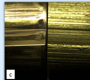
Figure 6: (a) Identifiable striations were observed from bullets fired from barrel A between 1<sup>st</sup> and 100<sup>th</sup> bullets; (b) Striations comparison between bullet fired from barrel A (left) and that from barrel B (right) resulted in an elimination of firing from the same barrel; (c) Obvious differences between the striations obtained from bullets fired from the conventional reference barrel (left) and that from the 3D-printed barrel A (right).
