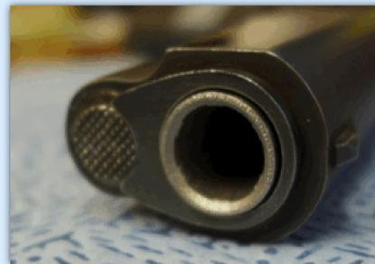
Figure 4: The final assembly of the barrel in the reference pistol after hand-fitting.
