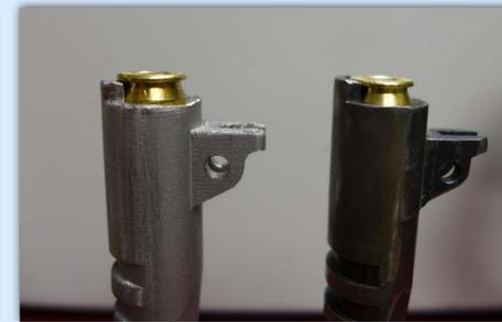
Figure 5: The cartridges were seated somewhat differently in the 3D-printed chamber (left) and on the reference chamber (right).
