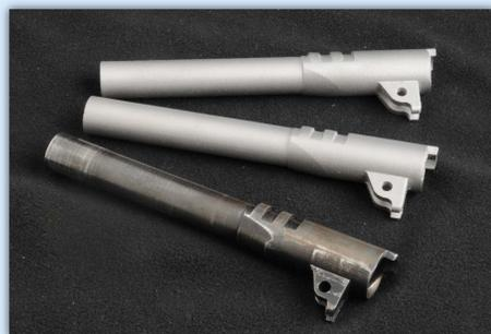
Figure 1: The two 3D-printed barrels are shown on the top and the bottom one is from a reference Colt 1911 45 Auto pistol.
