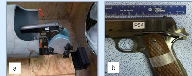
Figure 2: (a) The assembled pistol was secured in the ransom rest for test-firing; (b) The grip safety on the reference pistol was disengaged using a piece of tape before test-firing.
